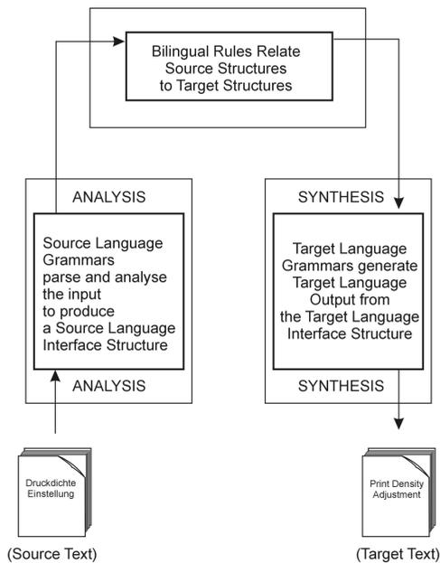
**Figure 5.3.** The architecture of a transfer-based system
