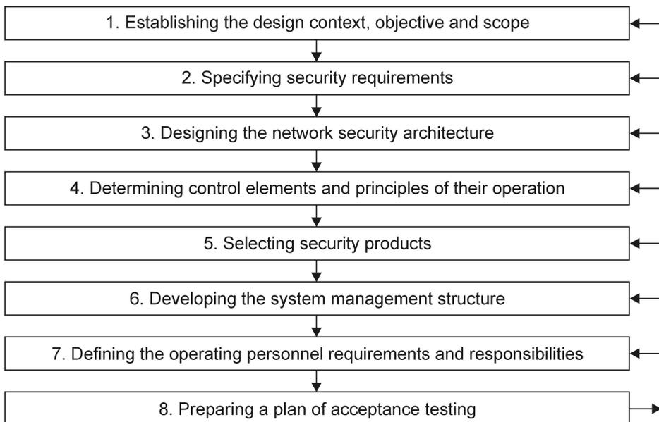
**Figure 17.1.** Stages of the security system designing
