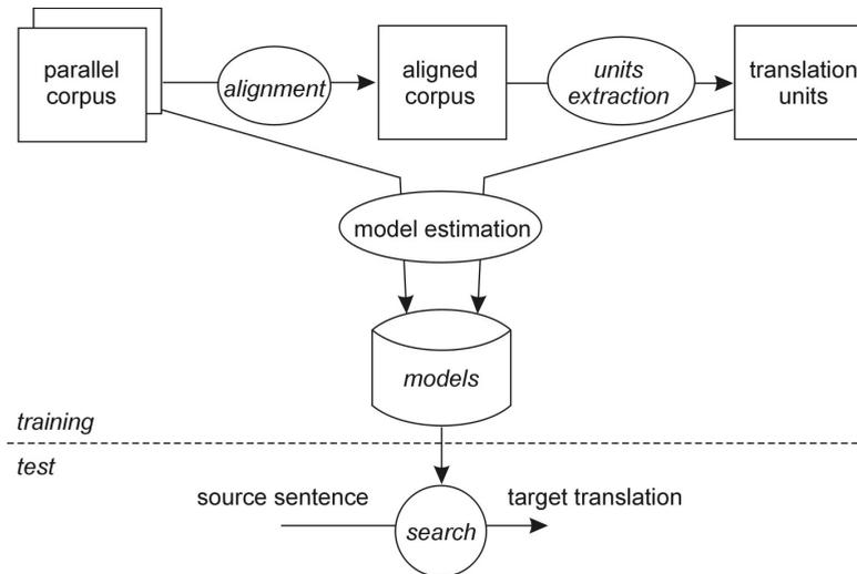
**Figure 5.5.** The architecture of statistical machine translation system
