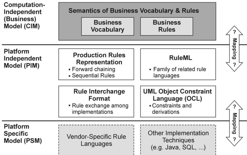
**Figure 15.1.** Model Driven Architecture layers
